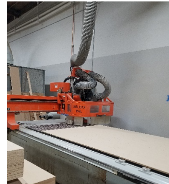
CNC machine cuts four doors at a time
