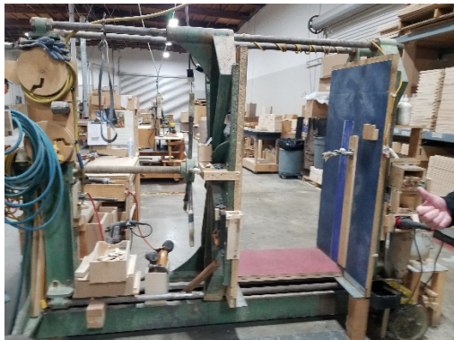
Original 1930's presses hold the Back-rail, bottom & sides when nailed and glued together
